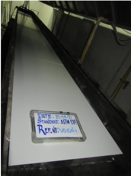
Photo 1: Specimen before the test. (Non-Fire Side)
