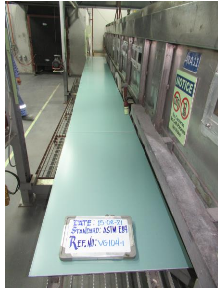
Photo 2: Specimen before the test. (Fire Side)
